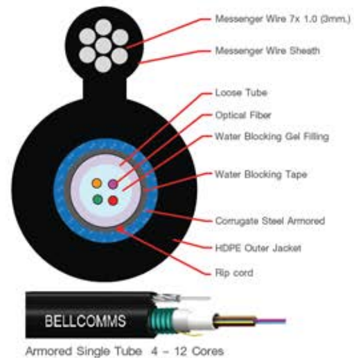
Armored Single Tube 4 - 12 Cores
